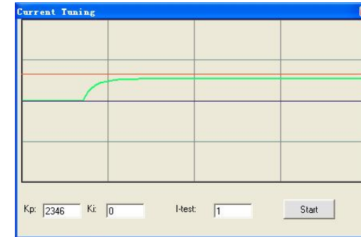
Figure 23: Kp=2346, Ki=0 (poor performances)
