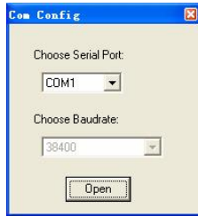
Figure 21: RS232 communication configuration window
