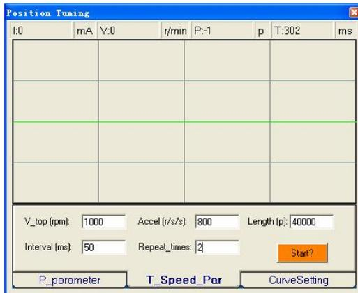
Figure 6-19: Self-test motion settings for the tuning
